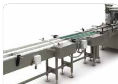
Automatic inline feeder for regular products
