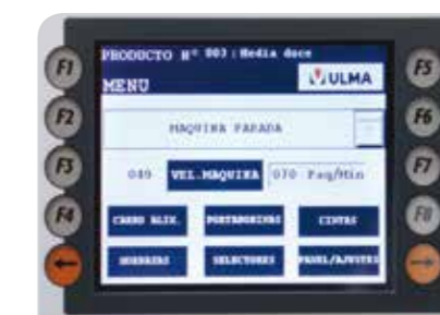
Touch screen control panel
