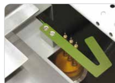
Ionizer for longitudinal sealing system
